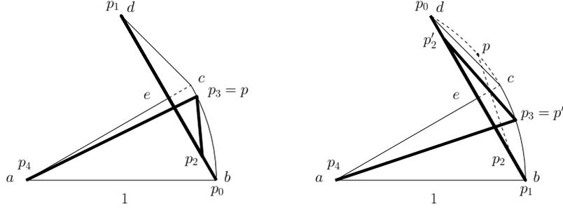
Figure 17: Folding of a 4-link ruler (in bold lines) into  $C2$ . Left:  $|p_2c| \leq x$ . Right:  $|p_2c| > x$ .
