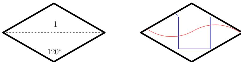
Figure 4: A universal case (in bold lines) for Moser’s worm problem. Left: a rhombus with a long diagonal of unit length and vertex angles of  $60^\circ$  and  $120^\circ$ . Right: two plane curves of length 1 contained in the case.
