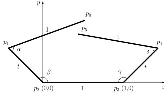
Figure 7: Legend for the 5-link ruler used (in bold lines). The figure does not show a valid folding, since e.g., the unit links do not pairwise intersect.
